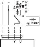
Control remotely 0...100% with positioner SG..
